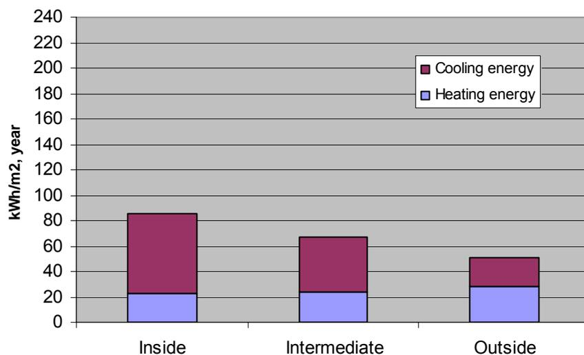
Figure 4.20 Calculated yearly energy use for heating and cooling for a reference building in Paris: Results for different positions of the shading devices (Venetian blinds). (i) inside the building; (ii) in an intermediate position between the glazed window panes; (iii) outside the building.
