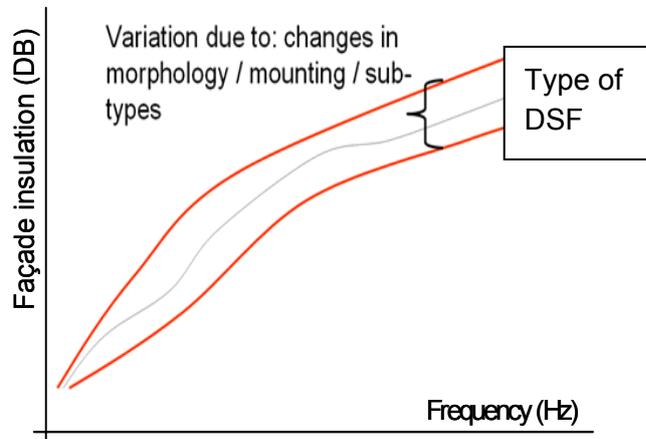
Figure 3.15 Façade sound insulation as function of frequency.
