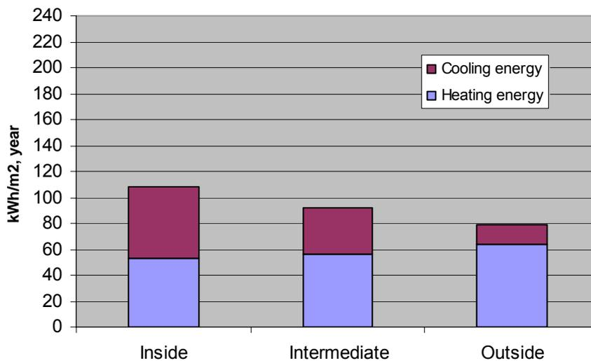
Figure 4.21 Calculated yearly energy use for heating and cooling for a reference building in Stockholm: Results for different positions of the shading devices (Venetian blinds). (i) inside the building; (ii) in an intermediate position between the glazed window panes; (iii) outside the building.
