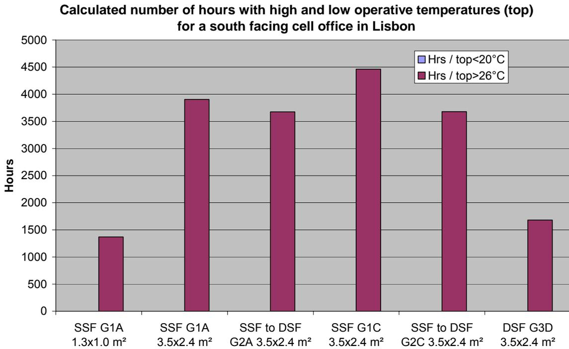
Figure 4.12 Calculated number of hours/year with high and low operative temperatures (top) for south facing cell office in Lisbon.
