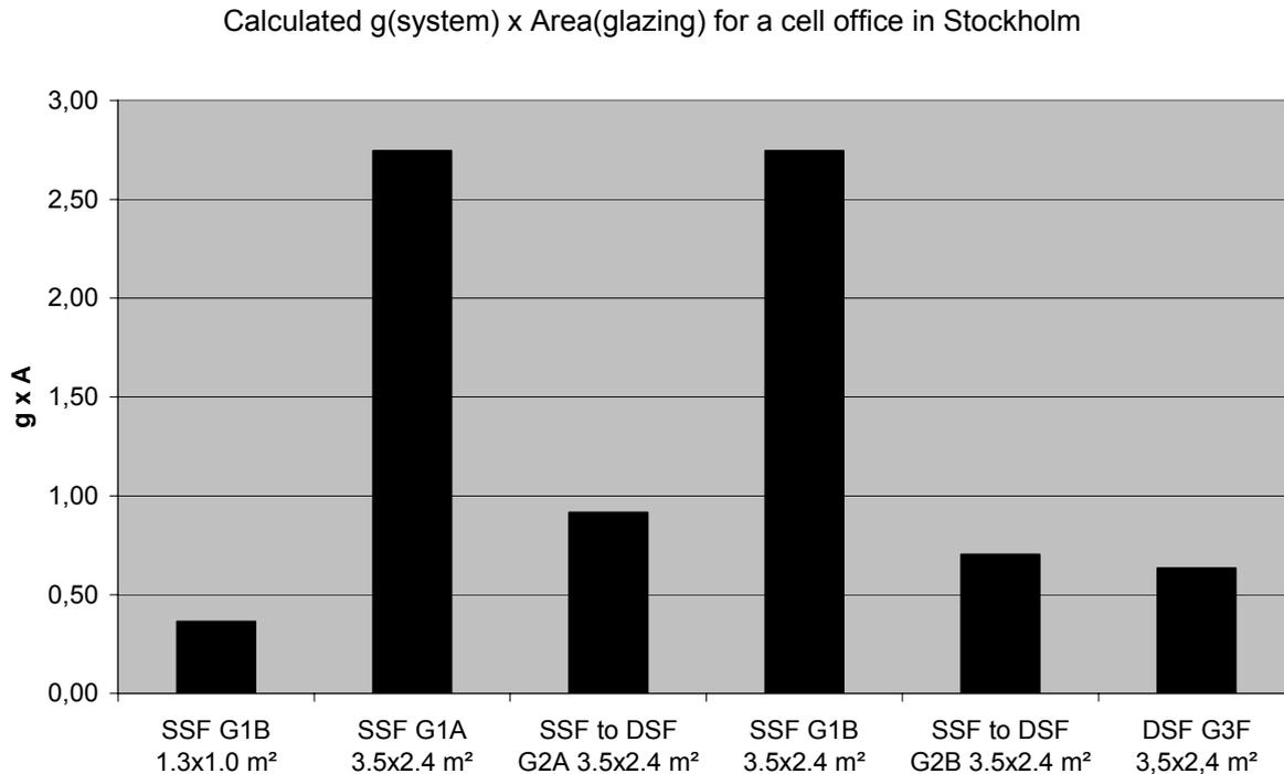
Figure 4.8 Calculated  $g_{\text{system}} \times \text{Area}_{\text{glazing}}$  for a south facing cell office in Stockholm.
