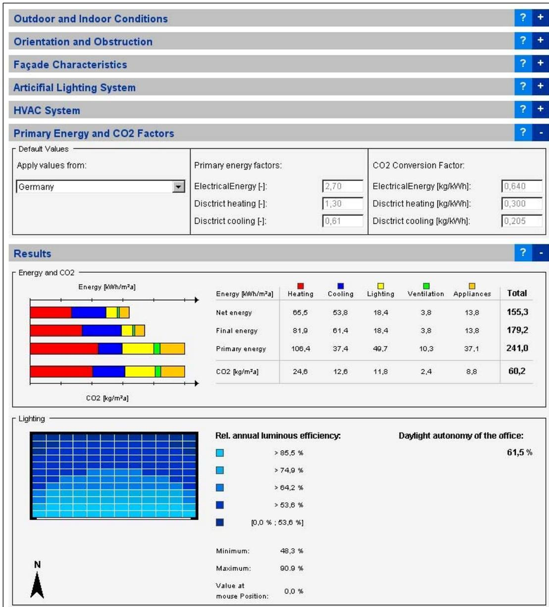
Figure. 5.7 Screenshot of the BESTFACADE tool part definition of the primary energy and CO<sub>2</sub> factors and results for energy, CO<sub>2</sub> and luminous efficiency and daylight autonomy.
