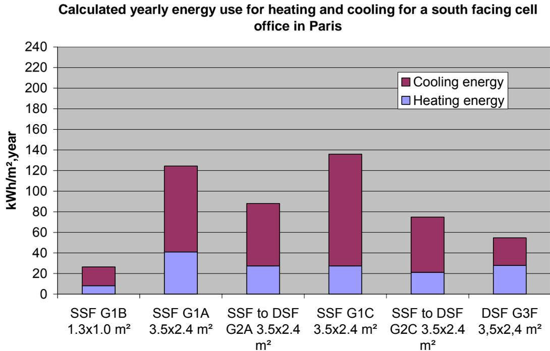
Figure 4.4 Calculated yearly energy use for heating and cooling for a cell office in Paris. The glazing types can be found in table 4.4 for SSF, table 4.5 for SSF to DSF and table 4.6 for DSF. SSF = single skin façade and DSF = double skin façade. SSF to DSF means retrofit of a single skin façade to a double skin façade.
