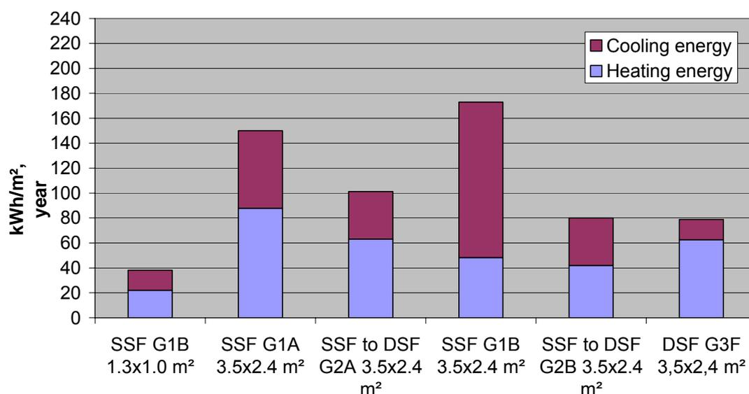
Figure 4.5 Calculated yearly energy use for heating and cooling for a cell office in Stockholm. The glazing types can be found in table 4.4 for SSF, table 4.5 for SSF to DSF and table 4.6 for DSF. SSF = single skin façade and DSF = double skin façade. SSF to DSF means retrofit of a single skin façade to a double skin facade.
