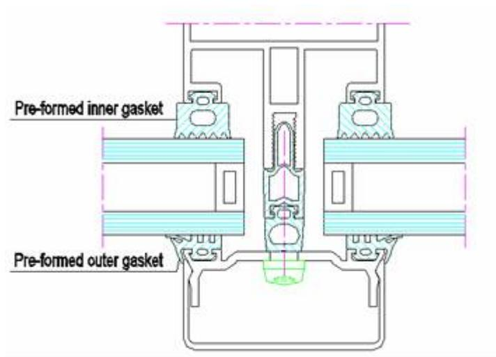
Figure 3. 21 Tightness of a glazed façade using inner and outer gaskets.
