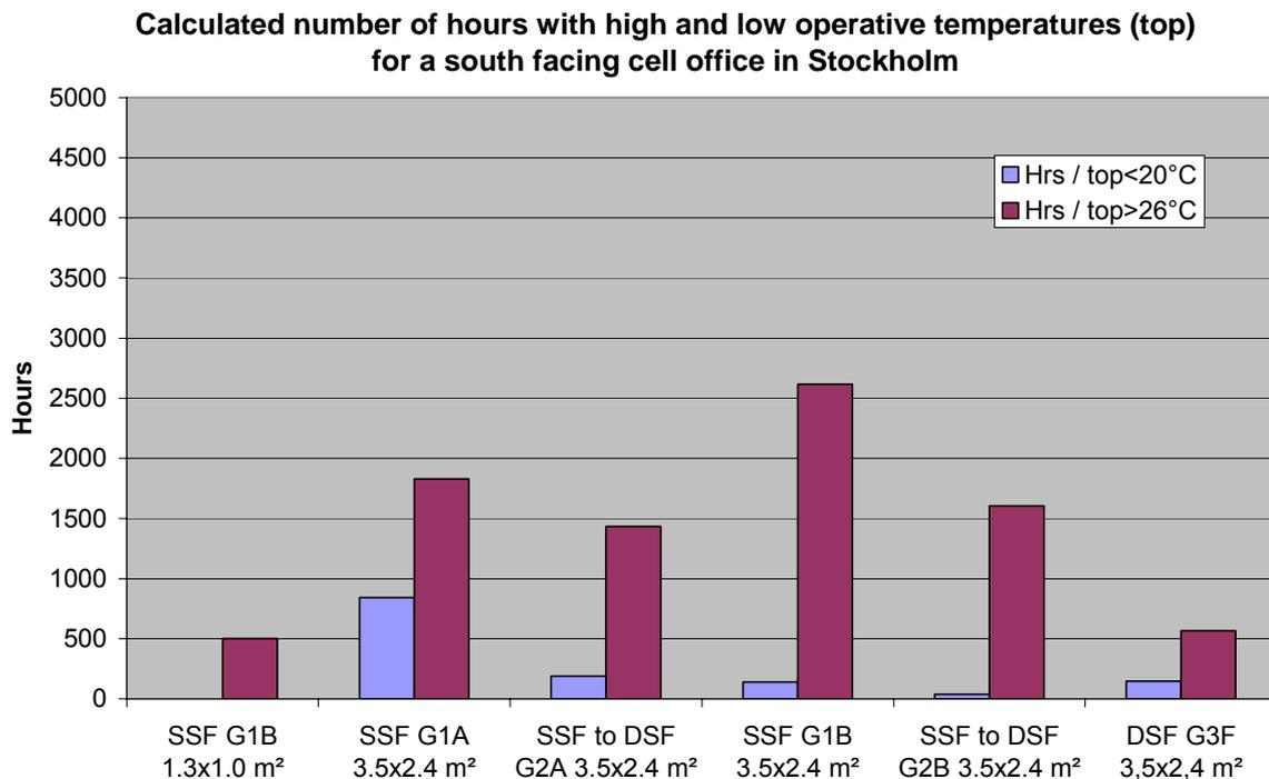
Figure 4.14 Calculated number of hours/year with high and low operative temperatures (top) for south facing cell office in Stockholm.
