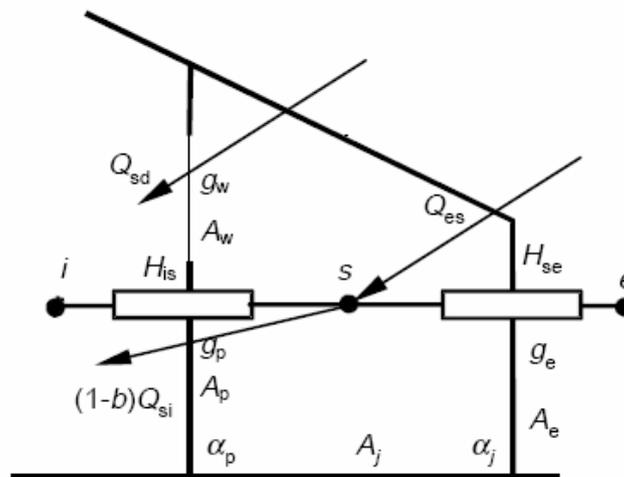
Figure 5.4 Scheme of the simple calculation method. The double skin façade is regarded as an attached sunspace. The scheme includes gains and heat loss coefficients and an equivalent circuit.
