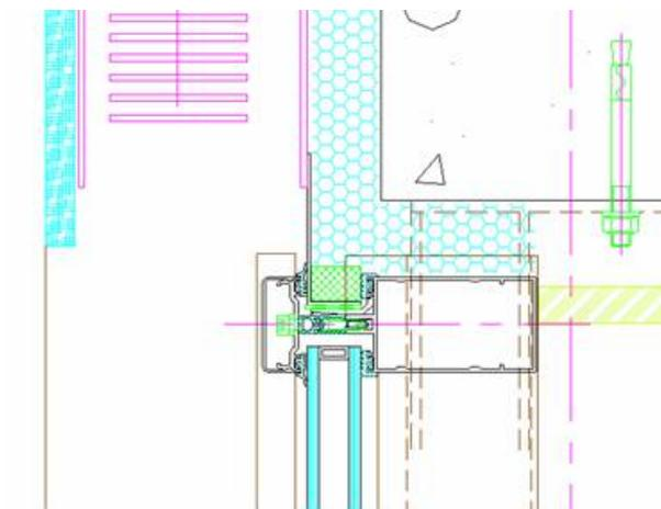
Figure 3.33 Section of the double glazed inner skin with standard curtain wall profiles
