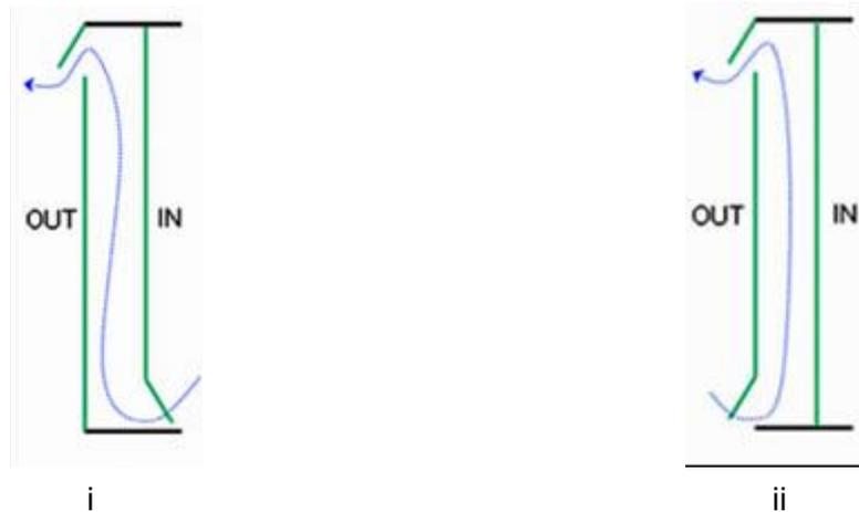
Figure 4.17 Ventilation of the air gap (i) Inside to Outside; (ii) Outside to Outside.
