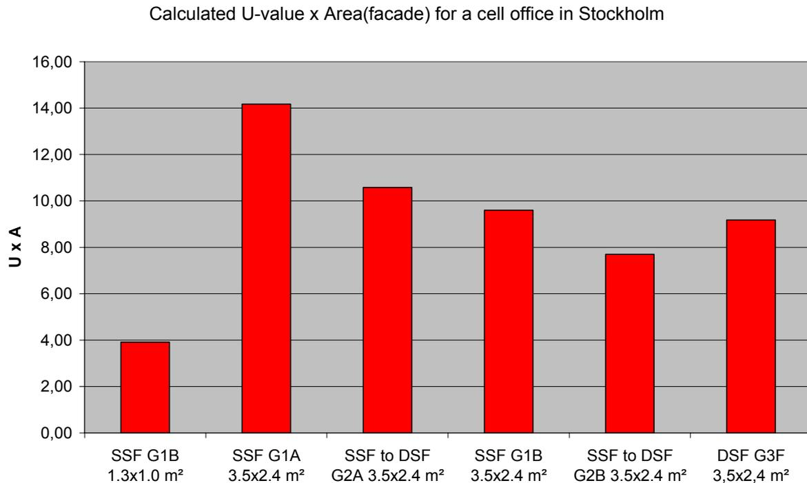
Figure 4.11 Calculated  $U_{\text{facade}} \times \text{Area}_{\text{facade}}$ , W/K, for a south facing cell office in Stockholm.
