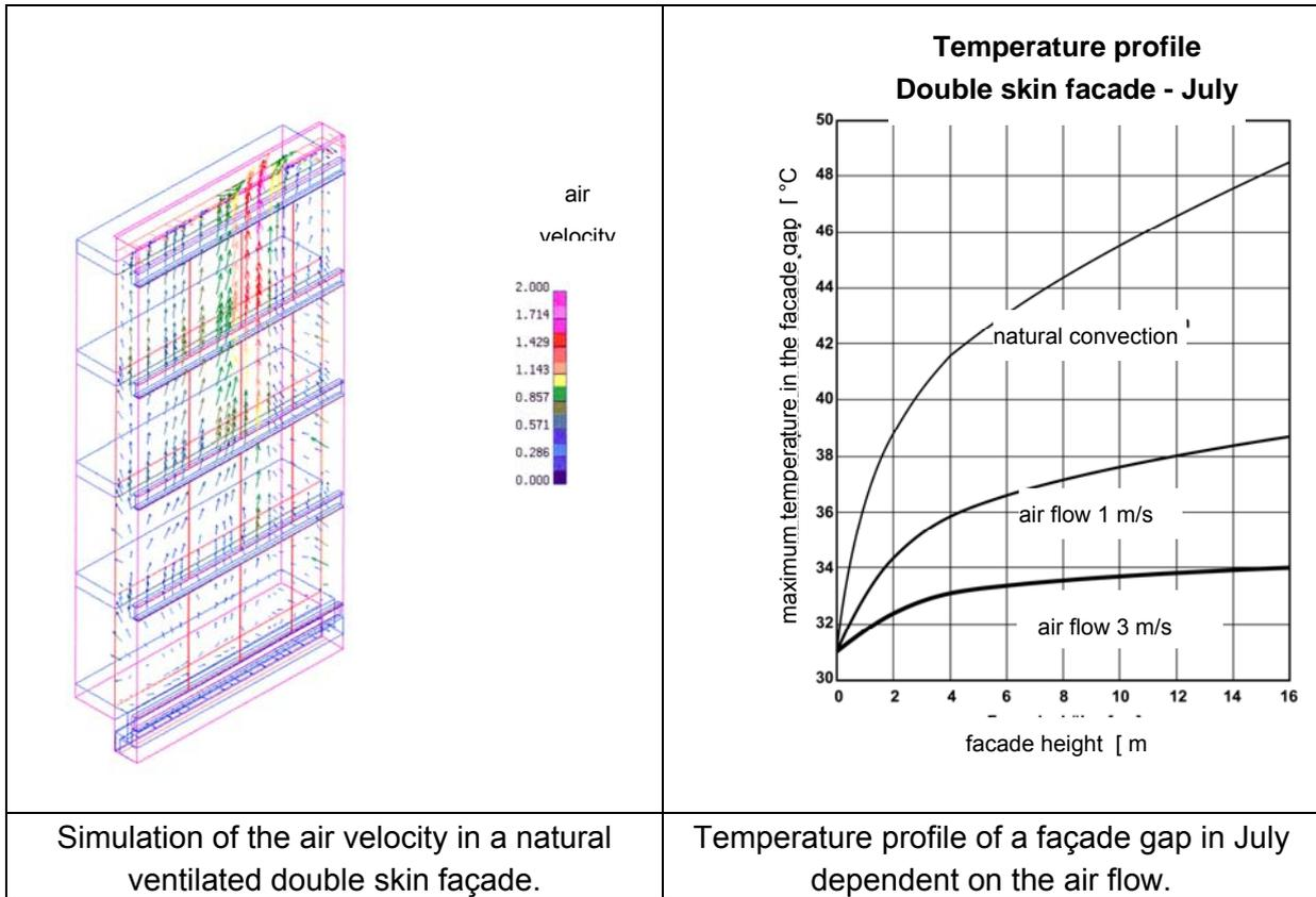
Figure 5.2 Examples for outputs of simulation tools for the energy performance of double skin facades.
