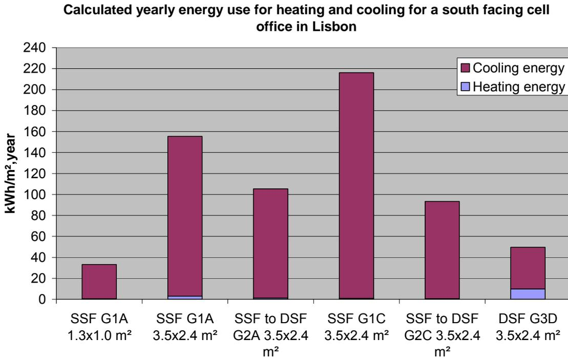
Figure 4.3 Calculated yearly energy use for heating and cooling for a cell office in Lisbon. The glazing types can be found in table 4.4 for SSF, table 4.5 for SSF to DSF and table 4.6 for DSF. SSF = single skin façade and DSF = double skin façade. SSF to DSF means retrofit of a single skin façade to a double skin facade.
