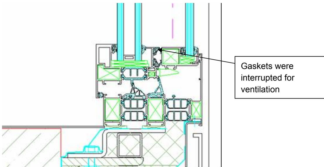
Figure 3.23 Detailed horizontal section of the window.
