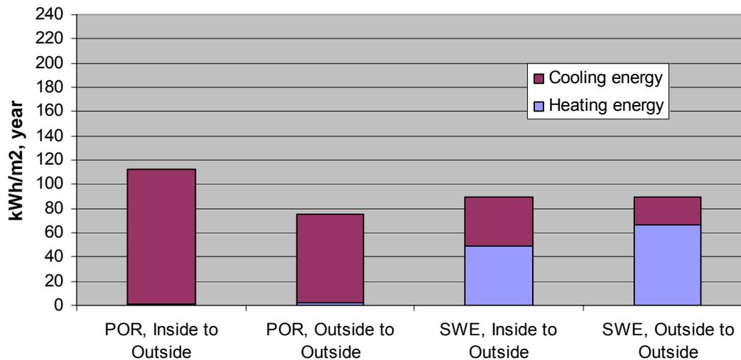
Figure 4.22 Calculated yearly energy use for heating and cooling for a reference building with a double skin façade in Lisbon (POR) and Stockholm (SWE): Results for different air gap ventilation strategies. Inside air to outside air and outside air to outside air.
