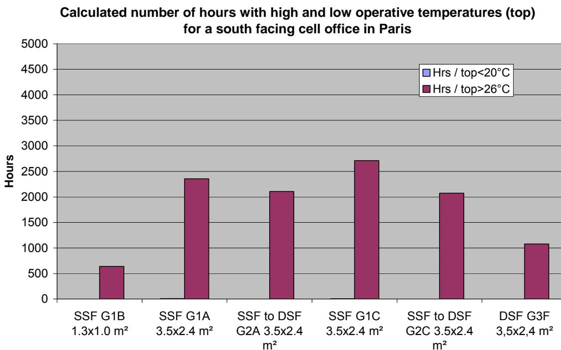
Figure 4.13 Calculated number of hours/year with high and low operative temperatures (top) for south facing cell office in Paris.
