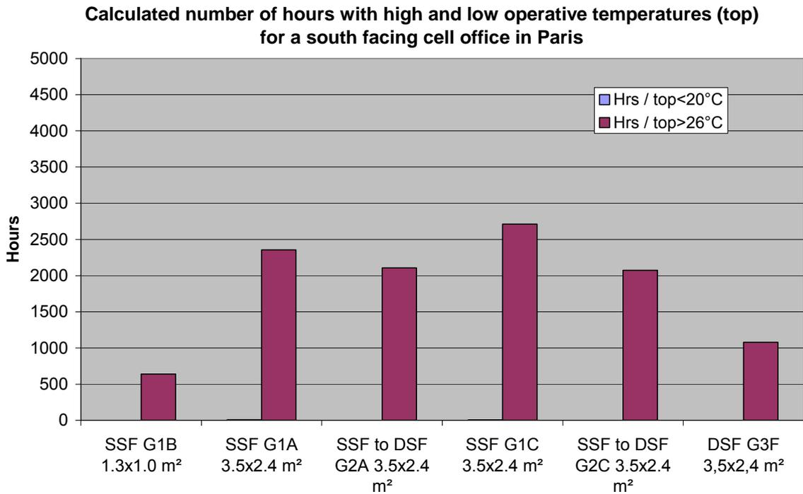
Figure 4.13 Calculated number of hours/year with high and low operative temperatures (top) for south facing cell office in Paris.
