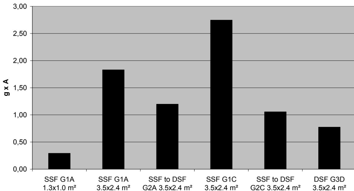
Figure 4.5 Calculated  $g_{\text{system}} \times \text{Area}_{\text{glazing}}$  for a south facing cell office in Lisbon.
