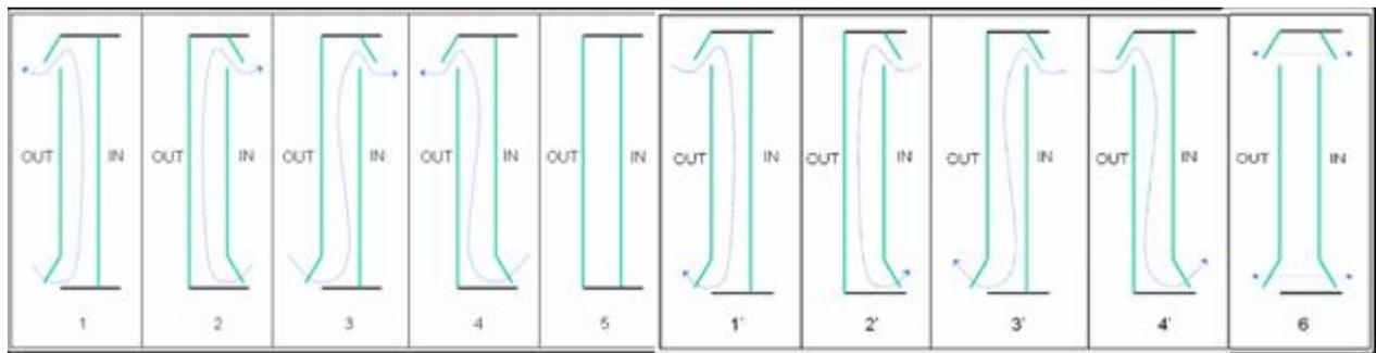
Figure 4.1 Ventilation mode variant for double skin façades.
