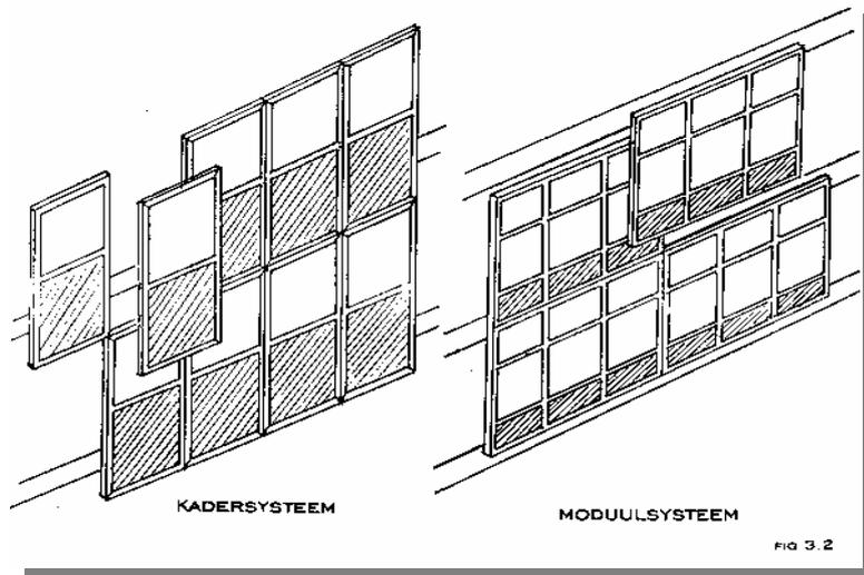
Figure 3.27 Combination of glass panels in element façade.
