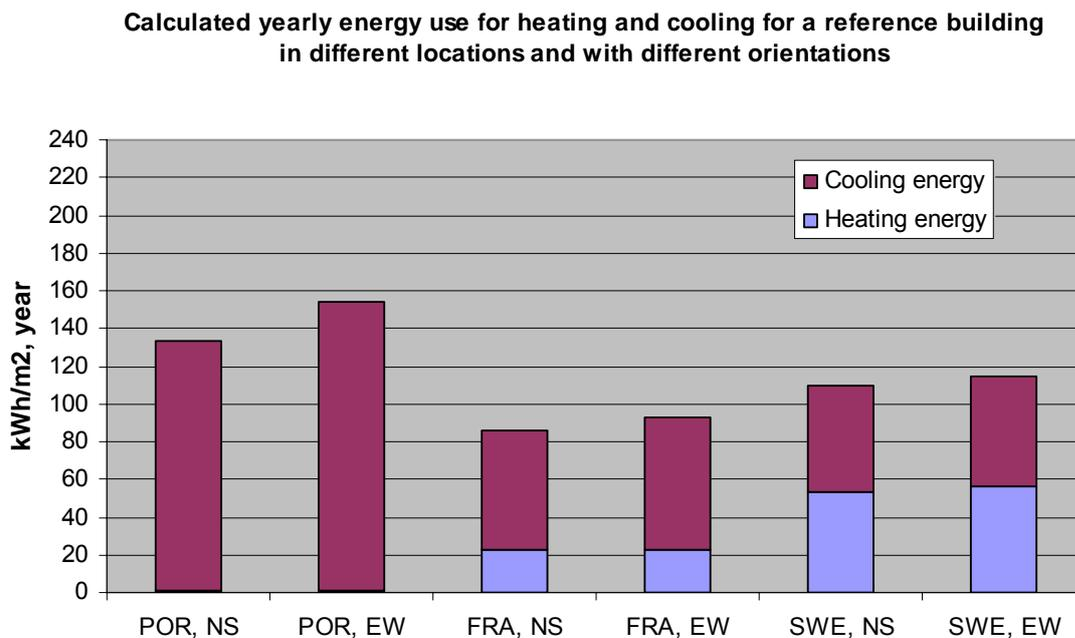
Figure 4.18 Calculated yearly energy use for heating and cooling for a fully glazed reference building located in Lisbon (POR), Paris (FRA) and Stockholm (SWE) with orientation North-South and East-West.
