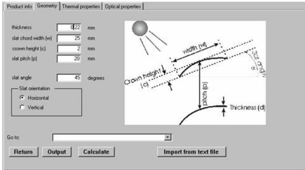
Figure 5.9 Geometrical definition of curved slat type blinds in WIS
