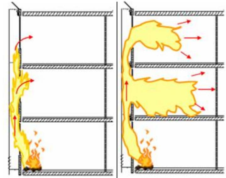
Figure 3.12 Propagation and penetration of the fire along a double skin facade
