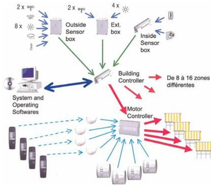
Figure 4.2 The different components for the control of shading devices (source: SOMFY)
