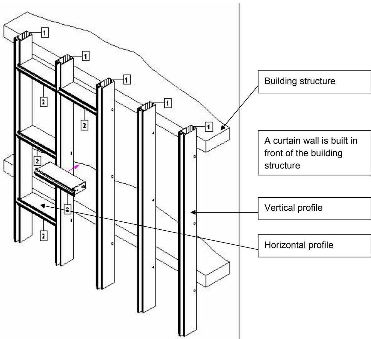
Figure 3.20 The principles of a curtain wall.
