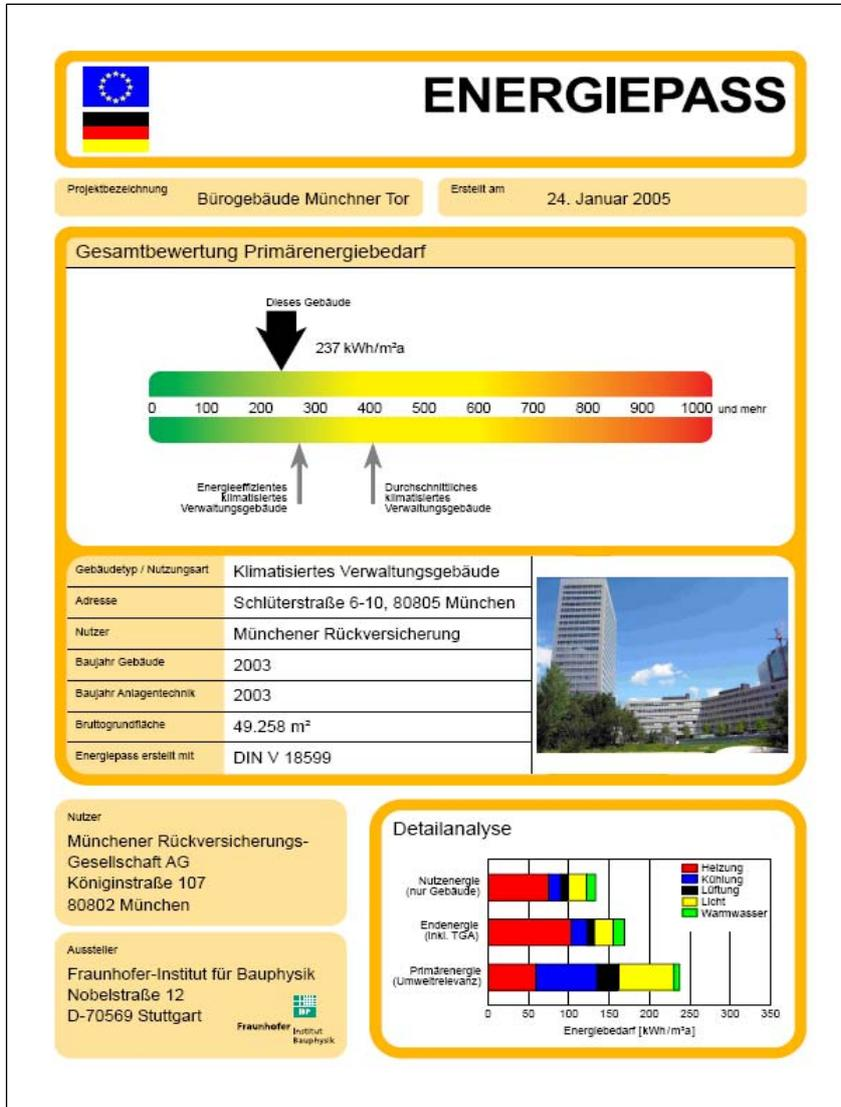
Figure 5.1 Energy performance certificate for a German double skin façade office building situated in Munich.
