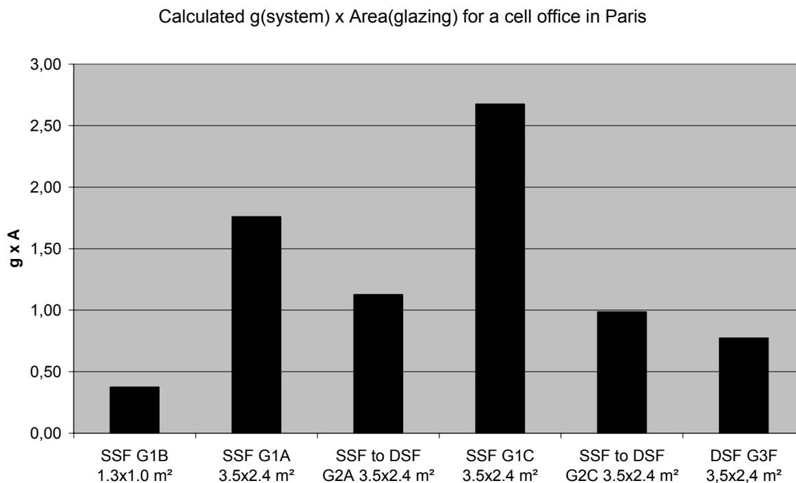
Figure 4.7 Calculated  $g_{\text{system}} \times \text{Area}_{\text{glazing}}$  for a south facing cell office in Paris.
