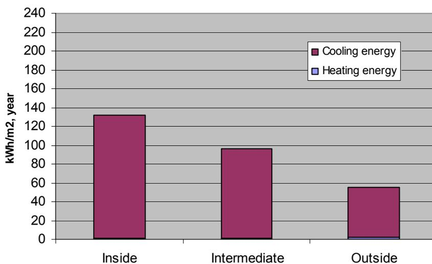
Figure 4.19 Calculated yearly energy use for heating and cooling for a reference building in Lisbon: Results for different positions of the shading devices (Venetian blinds). (i) inside the building; (ii) in an intermediate position between the glazed window panes; (iii) outside the building.
