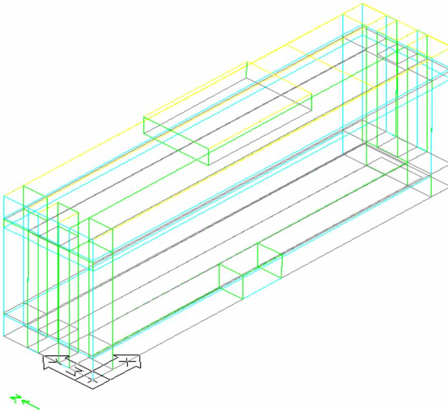
Figure 4.16 Model of the reference building and the thermal zones considered.
