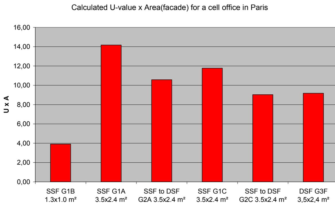
Figure 4.10 Calculated  $U_{\text{facade}} \times \text{Area}_{\text{facade}}$ , W/K, for a south facing cell office in Paris.
