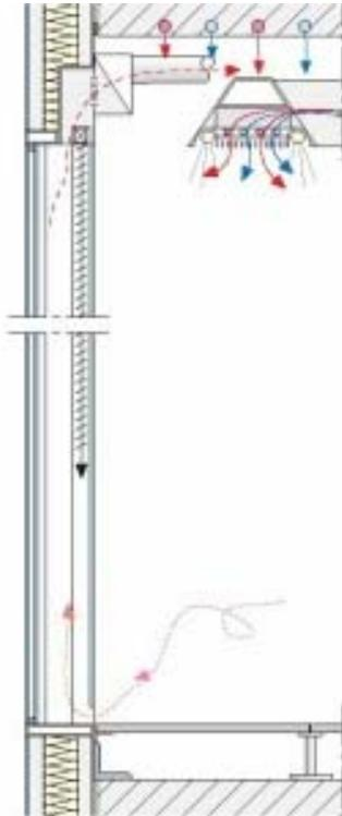
Figure 3.24 General extraction principle.
