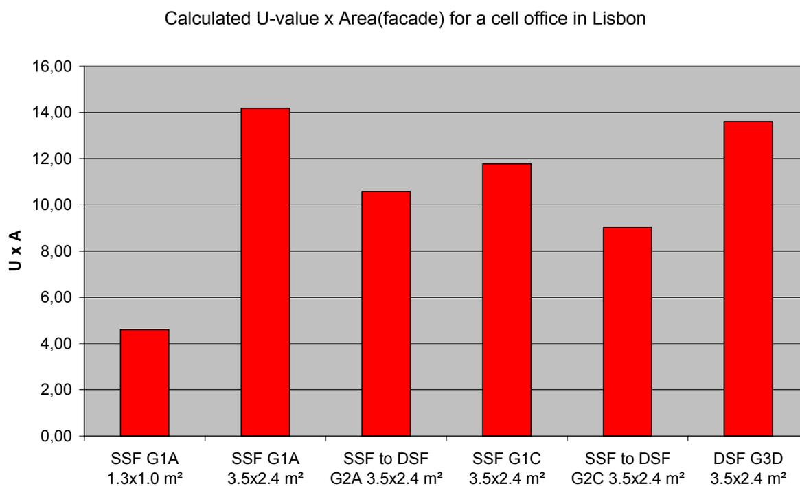
Figure 4.9 Calculated  $U_{\text{facade}} \times \text{Area}_{\text{facade}}$ , W/K, for a south facing cell office in Lisbon.
